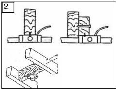
Before installing this fan make sure the outlet box is properly installed to the house structure. To reduce the risk of fire, electric shock, or personal injury, mount to outlet box or supporting system acceptable for fan support. (Mounting must support at least 35 lbs.(16 kg.)).
